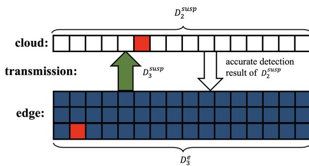
Figure 3. Data storage and transmission for round 3 of the proposed cloud–edge collaboration.
