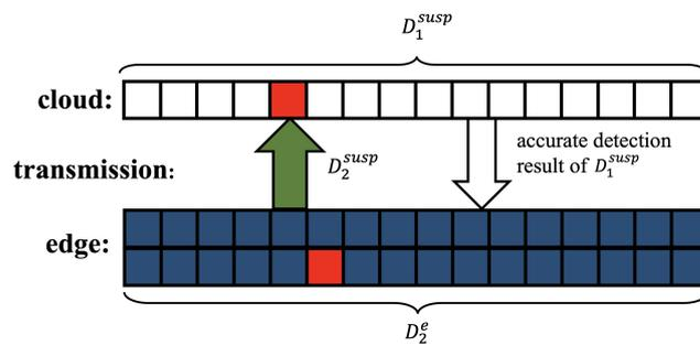
Figure 2. Data storage and transmission for round 2 of the proposed cloud–edge collaboration.
