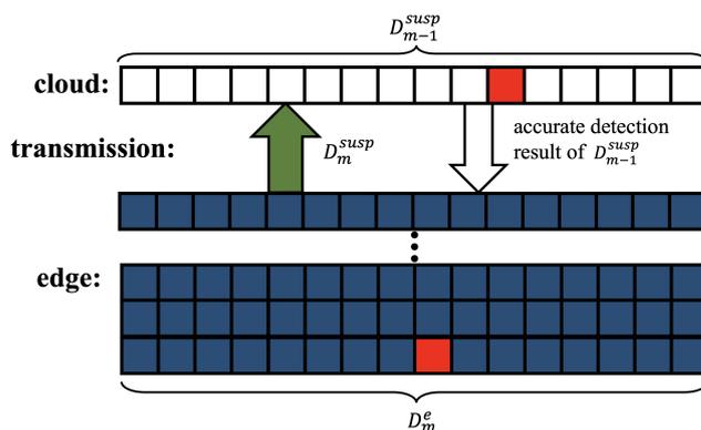
Figure 4. Data storage and transmission for round  $m$  of the proposed cloud–edge collaboration.
