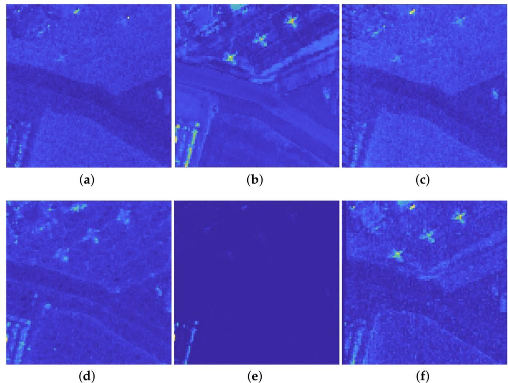
**Figure 9.** Detection performance of different algorithms for real-data1. (a) CLP-RX Algorithm; (b) LRASR Algorithm; (c) RGAE Algorithm; (d) LSUNRSOR Algorithm; (e) FEBP Algorithm; (f) CE-RX Algorithm.
