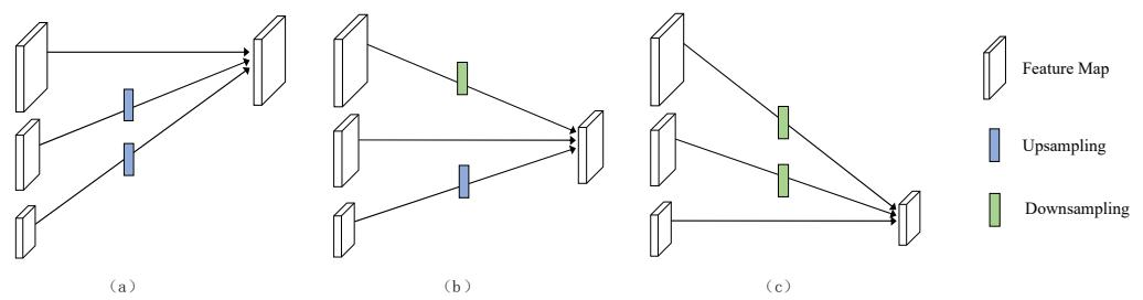
**Figure 3.** Multi-branch feature fusion process. (a) represents the 1/4 branch fuse feature information from the 1/8 and 1/16 branches, (b) represents the 1/8 branch fuse feature information from the 1/4 and 1/16 branches, and (c) represents the 1/16 branch fuse feature information from the 1/4 and 1/8 branches.
