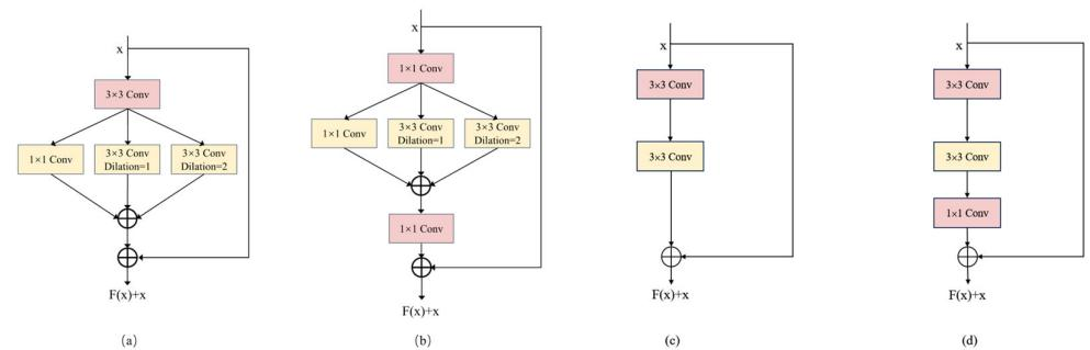
**Figure 4.** Structure of the multi-scale feature representation module. (a) denotes the module based on the BasicBlock unit, (b) denotes the module based on the BottleNeck unit, (c) denotes the original BasicBlock unit, and (d) denotes the original BottleNeck unit.
