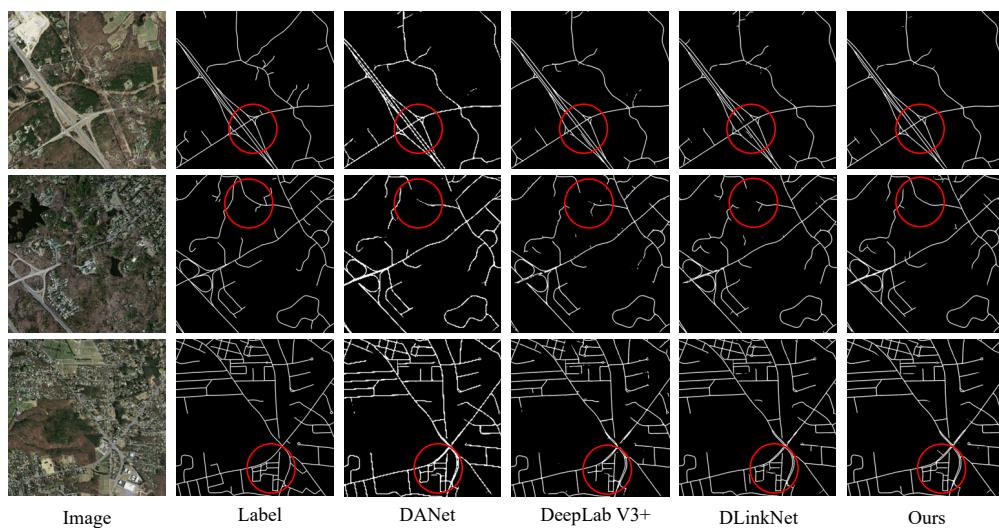
**Figure 7.** Qualitative evaluation results on the Massachusetts dataset. Each image covers an area of 1800 m × 1800 m.
