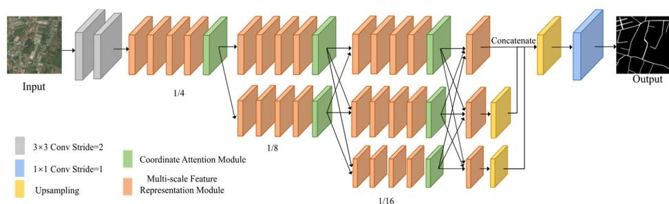
**Figure 2.** Specific structure of the CR-HR-RoadNet.
