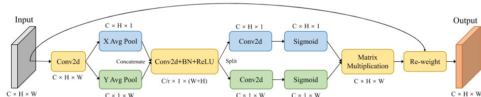
**Figure 5.** Structure of the coordinate attention module. For a detailed explanation, please refer to Section 3.3.
