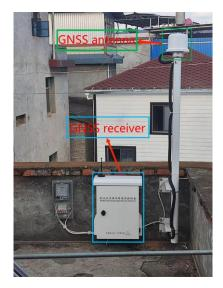
Figure 3. Data acquisition equipment.
