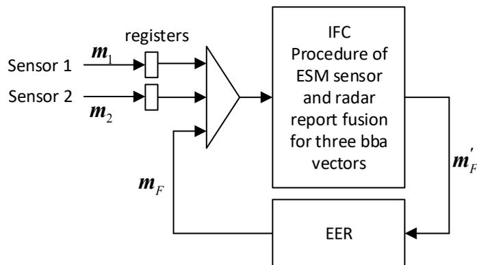
**Figure 3.** The diagram of the information-fusion process in the information-fusion center (IFC) for two sensors and electronic entity record from the IFC database. Explanations:  $m_i$ , a BBA measure vector of  $i$ -th sensor;  $m_F$ , a generalized BBA measure vector that is a part of the electronic entity record in the IFC; EER, an electronic entity record in the IFC database.
