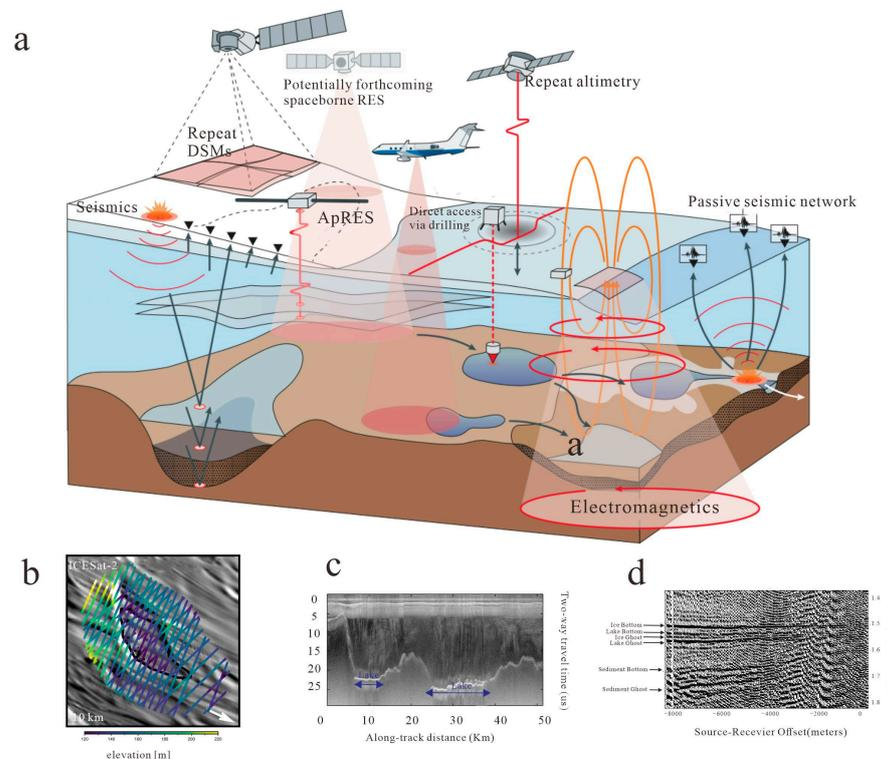
**Figure 8.** (a) Main geophysical methods for detecting subglacial hydrology [206]; (b) ICESat-2 altimetry coverage of active subglacial lakes in Antarctica [213]; (c) Radargrams of the Antarctic subglacial hydrological environment [214]; (d) The subglacial lake was imaged using seismic data [215].
