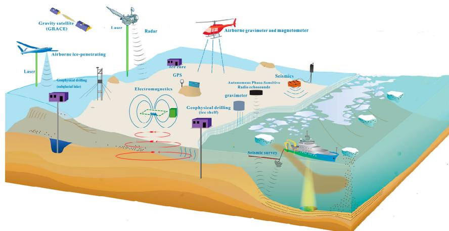
**Figure 6.** Geophysical observation methods applied to the Antarctic ice sheet (modified from [118]).
