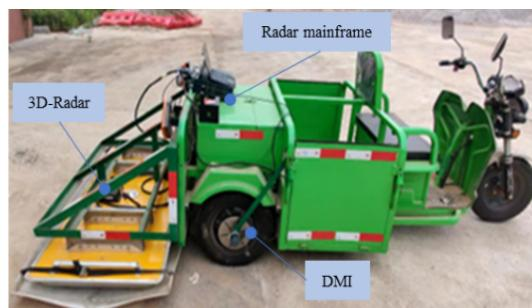
**Figure 9.** GPR data acquisition equipment.
