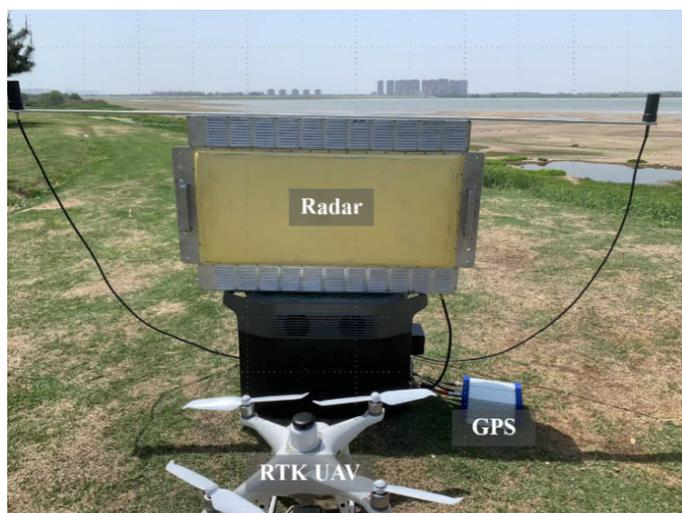
**Figure 18.** The experimental equipment consists of a radar, UAV, and GPS.
