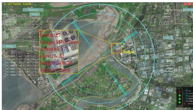
**Figure 17.** The detection result shown in P Type Radar Indicator.
