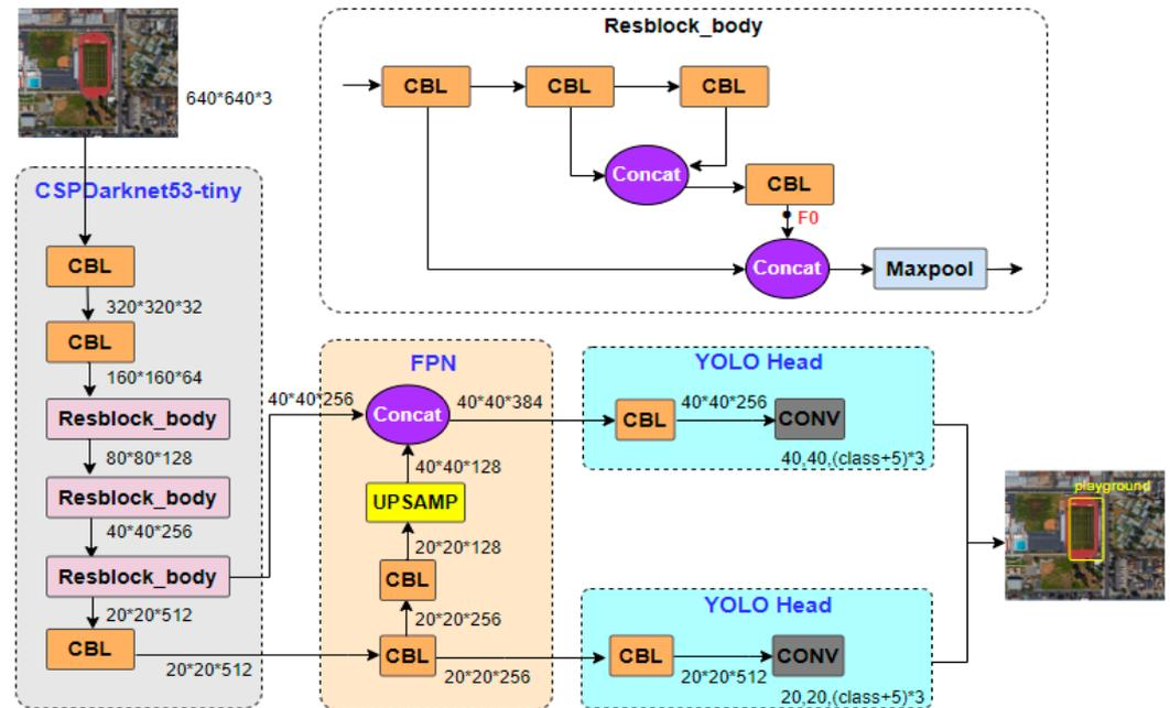
Figure 2. Structure of YOLOv4-tiny.
