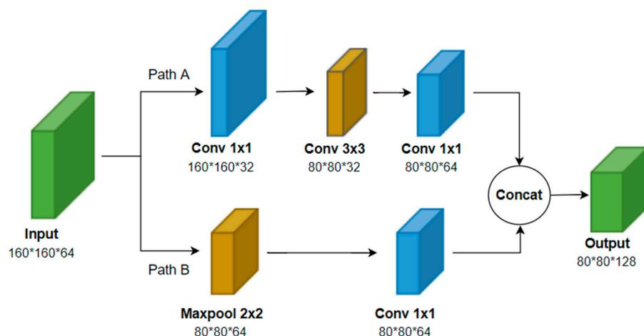
Figure 7. Structure diagram of Resblock\_M.
