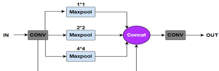
Figure 3. Structure of SPP.
