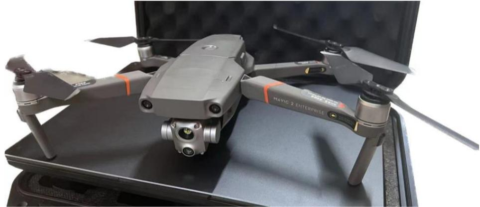
**Figure 1.** Exterior view of the UAV. The UAV is equipped with visible and infrared cameras and can capture images from the same angle and position simultaneously.
