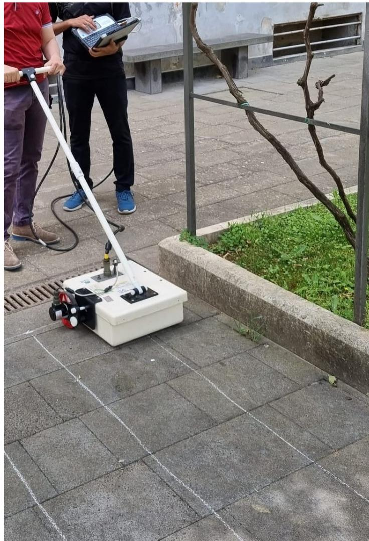
**Figure 4.** Photo of the IDS RIS-K2 Georadar system used to collect the scattered field measurements.
