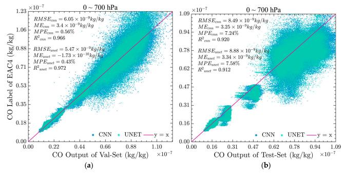
Figure 9. Scatter plot of model retrieval for CO (0~700 hPa): (a)val set; (b) test set.
