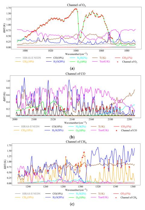
Figure 4. The preferred channel of atmospheric component gases. (a) O<sub>3</sub> (b) CO (c) CH<sub>4</sub>.
