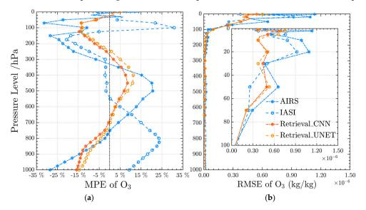
**Figure 13.** Comparison of O<sub>3</sub> between retrieval results and similar satellite products: (a) MPE; (b) RMSE.
