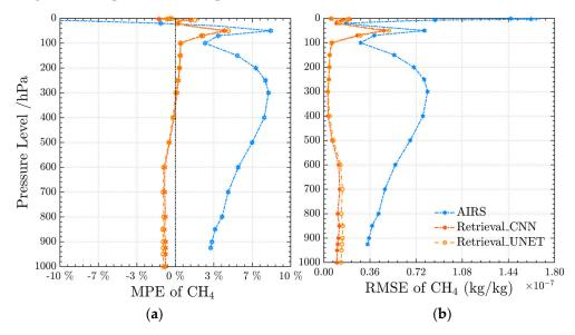
**Figure 19.** Comparison of  $CH_4$  between retrieval results and similar satellite products (a) MPE (b) RMSE.
