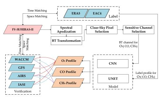
Figure 1. Retrieval system for gases profiles by FY-3E/HIRAS-II.
