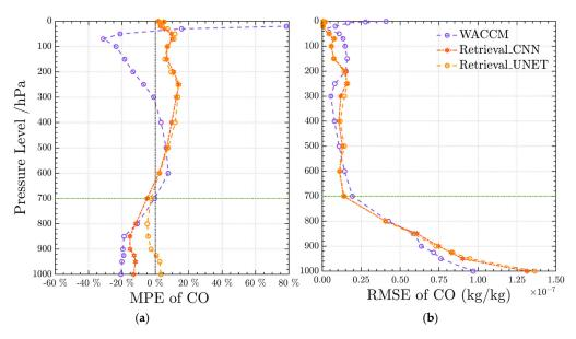
Figure 15. Comparison of CO between retrieval results and forecast data: (a) MPE; (b) RMSE.
