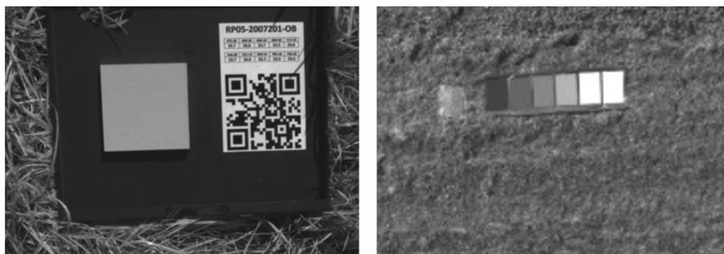
**Figure 2.** **Left:** white reference panel captured in band 5 (642 nm–658 nm) of the MicaSense dual camera system. **Right:** Aerial image of the 6 RRTs captured in band 2 (459 nm–491 nm).
