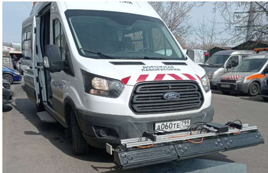
Figure 4. The arrangement of the radar antenna array on the road laboratory vehicle of the Russian Road Research Institute.
