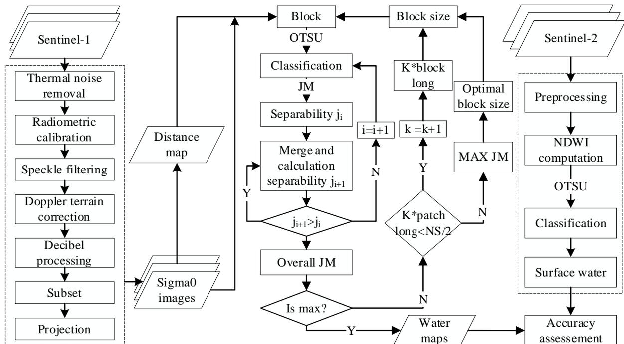
**Figure 2.** Workflow of the proposed method.
