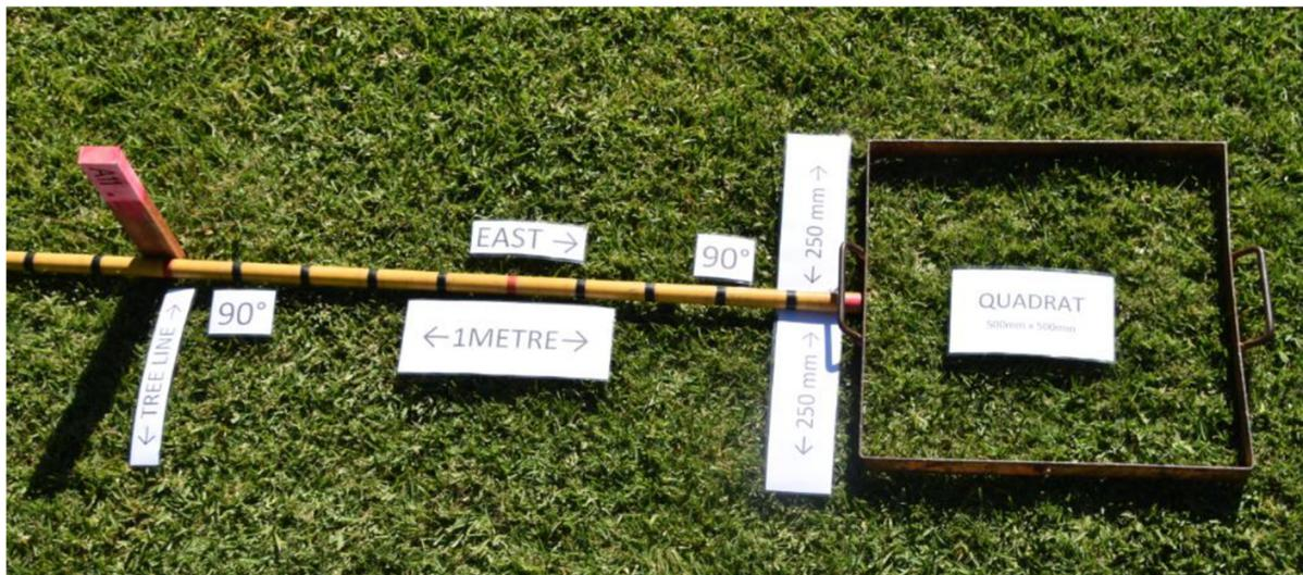
**Figure 2.** Illustration of the method used to position the quadrat relative to labelled stake.
