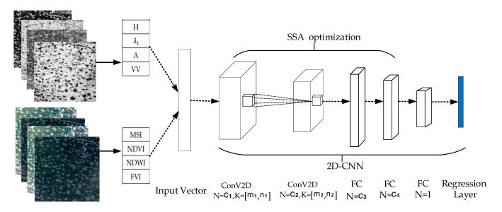
Figure 4. Structure of the proposed SSA-CNN model.
