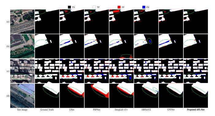
**Figure 12.** (**a**–**d**) Sample building segmentation results from the selected models with the BITCC dataset (comparative experiment).
