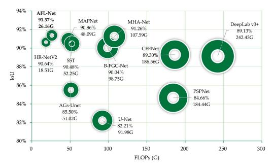
**Figure 14.** Comparison of the accuracy and complexity of selected models, annotated with IoU and computational cost in each model.
