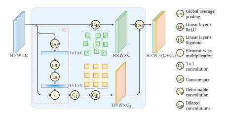
**Figure 4.** Structure diagram of the SFR module. Deformable convolution and dilated convolution expand the receptive field.
