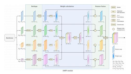
**Figure 2.** Schematic diagram of the AMFF module structure. The attention mechanism facilitates adaptive adjustment of the weights of the distinctive features.
