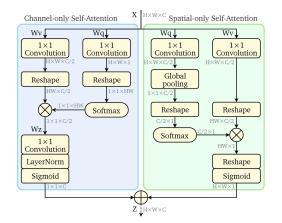
**Figure 3.** Structure diagram of attention mechanism in the AMFF module. Attentional weights are calculated at the channel and spatial dimensions.
