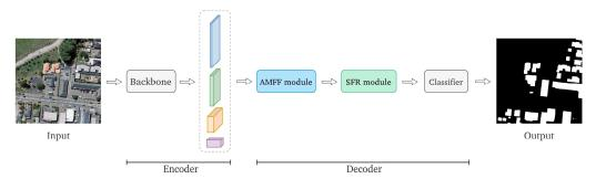
**Figure 1.** Schematic diagram of the AFL-Net framework. The encoder extracts the features through the backbone, outputting four feature maps at different scales. The decoder fuses the feature maps via the AMFF module, optimizes the building shape features via the SFR module, and outputs the building segmentation mask after the classifier.
