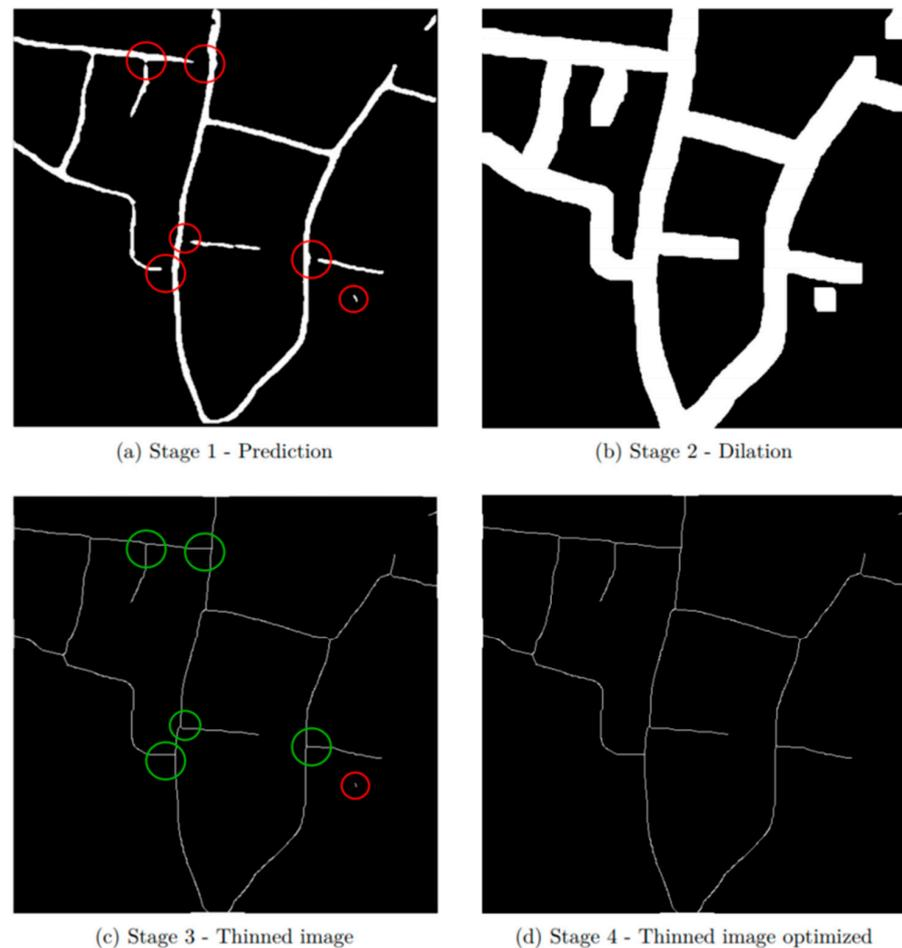
**Figure 6.** Sample results of road connection optimization process: (a) stage 1—prediction (red circles represent missing intersections and an artifact); (b) stage 2—dilation; (c) stage 3—thinning (the intersections in green circles have been corrected; the artifact in the red circle is going to be removed); (d) final results after removing smaller objects.
