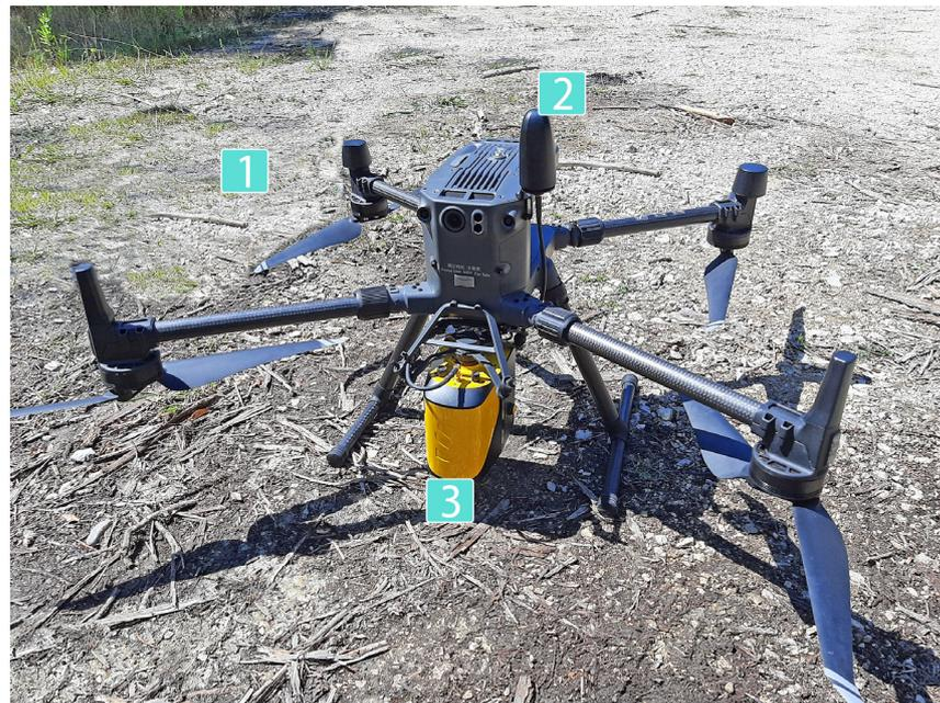
**Figure 3.** Unmanned aerial vehicle (UAV) used to collect LiDAR point clouds: (1) Matrice 300 RTK; (2) YellowScan RTK Antenna; (3) YellowScan Mapper.
