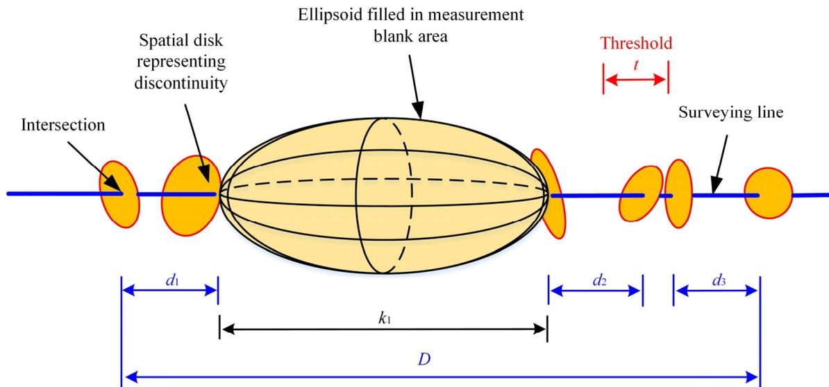
**Figure 5.** Determining RQD of a single surveying line, which eliminates influence of measurement blank area.
