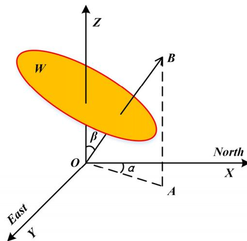
Figure 4. Three-dimensional representation of discontinuity.
