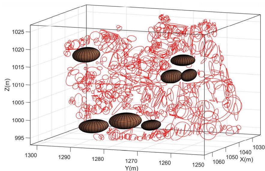
**Figure 6.** Three-dimensional disk model of discontinuities with ellipsoids.
