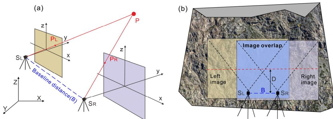
**Figure 2.** (a) Principle of digital close-range photogrammetry; (b) Schematic diagram of photograph perpendicular to slope.
