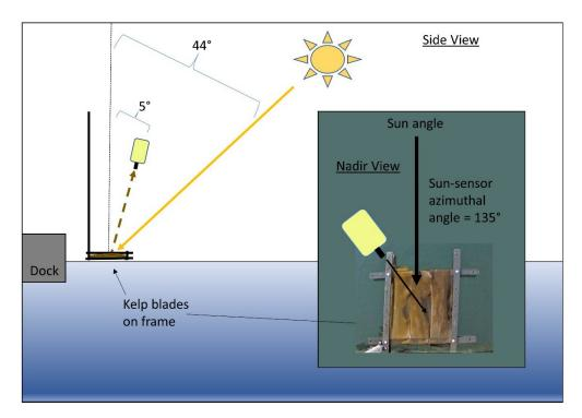
**Figure 1.** Side view of submergence experiment showing the geometry of acquisition for spectroradiometer and angle of zenith for the sun. Inset shows nadir view of the experiment with the azimuthal angle between spectroradiometer and sun and kelp blades inside the black frame. Diagrams are not to scale.
