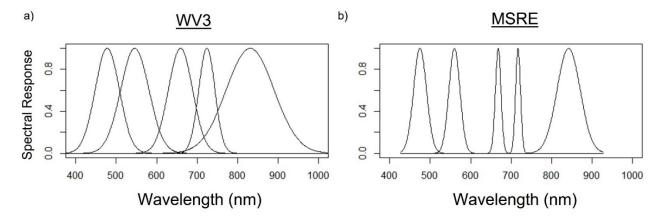
**Figure 2.** Relative spectral responses at each band according to Gaussian functions were used to simulate the shared bands of (a) WorldView-3 (WV-3) earth observation satellite and (b) Micasense RedEdge-MX (MSRE) uncrewed aerial vehicle sensors—from left to right: blue, green, red, red-edge, and near-infrared band locations are shown.
