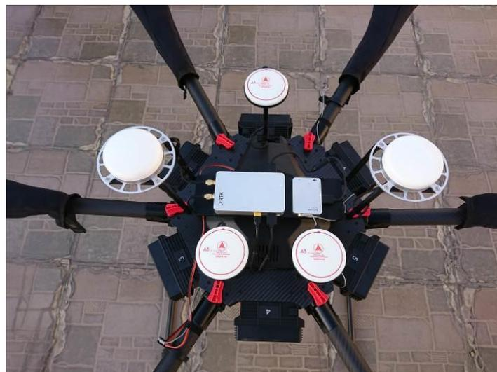
**Figure 6.** The DJI M600 UAV with a dual-antenna D-RTK kit installed.
