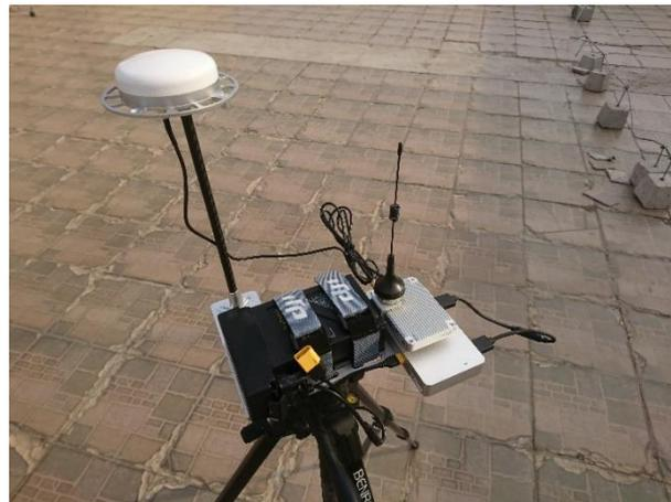
**Figure 7.** The differential ground station of the D-RTK suite.
