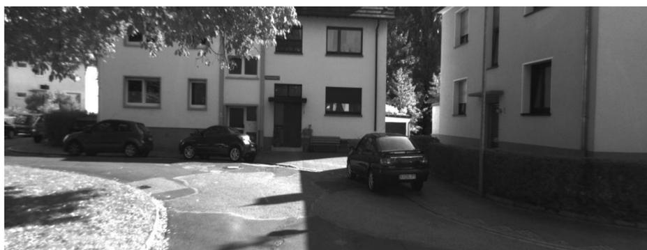
**Figure 7.** Typical obscured scene. The buildings in the figure and also the shade of trees can block the GPS signal propagation and affect the performance of RTK.
