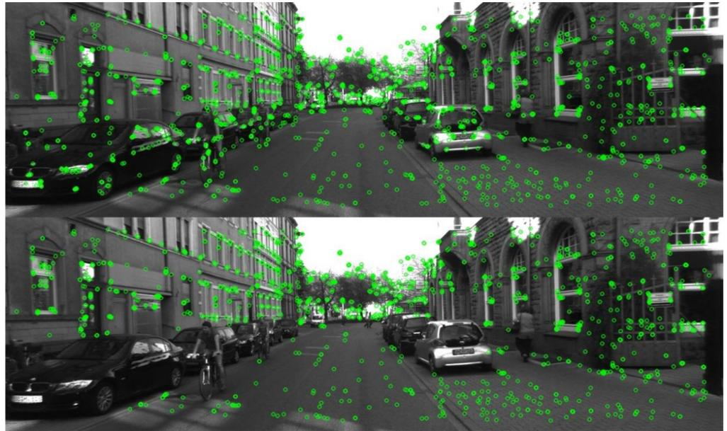
**Figure 8.** Feature image before and after excluding features on dynamic objects. The above image is the result extracting features using ORB-SLAM2. The below image is the result extracting features using Dynamic-SLAM. In the below image, dynamic objects like pedestrian, bicycle and car are segmented out, on which there are no feature points.
