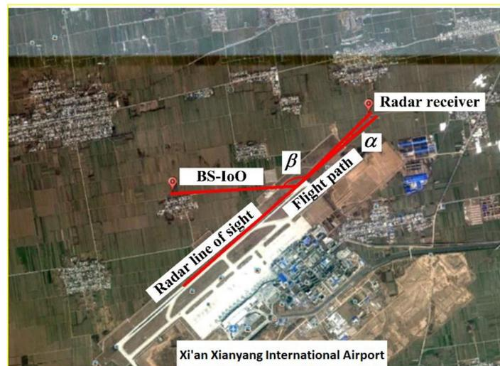
Figure 14. Sketch of radar setup.
