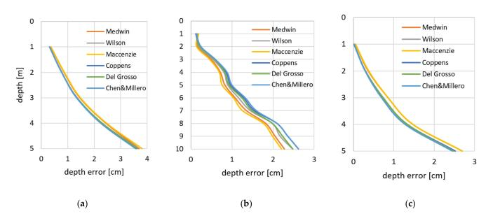
Figure 12. Depth error for measurements in the Motława (a) and Martwa Wisła (b) Rivers and Gdynia (c).
