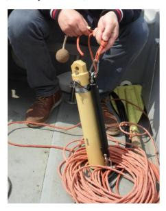
Figure 3. STD/CTD probe model SD204.
