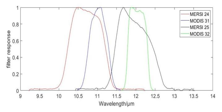
Figure 1. MERSI (channels 24 and 25) and MODIS (channels 31 and 32) central wavelengths at 11  $\mu$ m and 12  $\mu$ m spectral response function.
