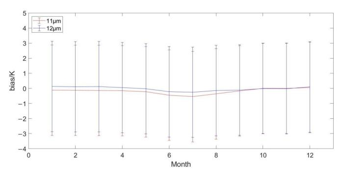
**Figure 9.** Mean bias and Std of the thermal infrared channels 11  $\mu$ m and 12  $\mu$ m  $T_b$  data for MERSI and MODIS.
