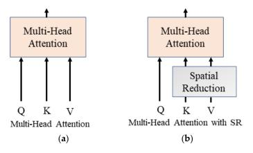
**Figure 2.** Structure of attention. ((**a**) is the multi-head attention of vanilla transformer and (**b**) is the multi-head attention with spatial reduction of transformer).
