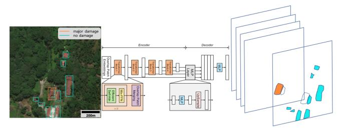
**Figure 5.** Overall model structure of SegDetector, which is based on SegFormer, to implement sub-channel target detection.
