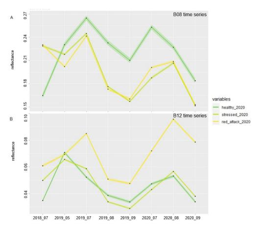
**Figure 5.** Mean seasonal B08 (**A**) and B12 (**B**) band reflectance (line) and standard error from 95% CI (confidence band) in a time series from 2018 to 2020 for healthy, stressed and red-attack stage canopies using training data from 2020.
