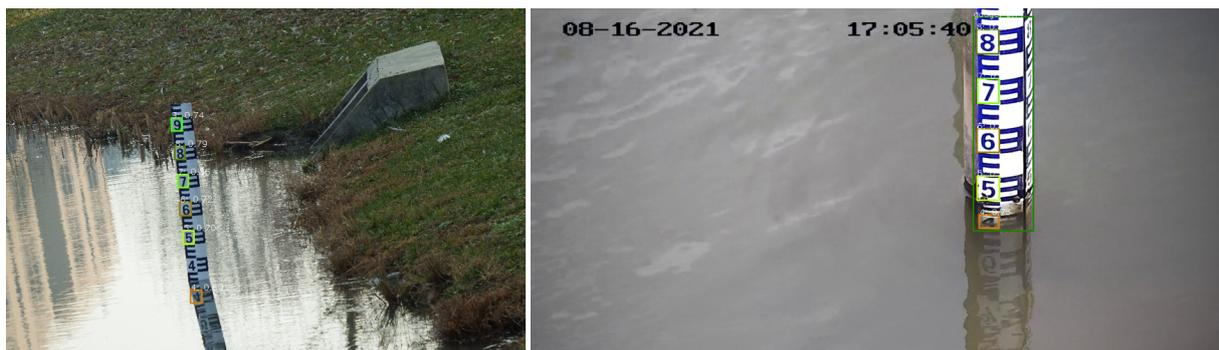
**Figure 7.** Inverted water gauge image detection results.
