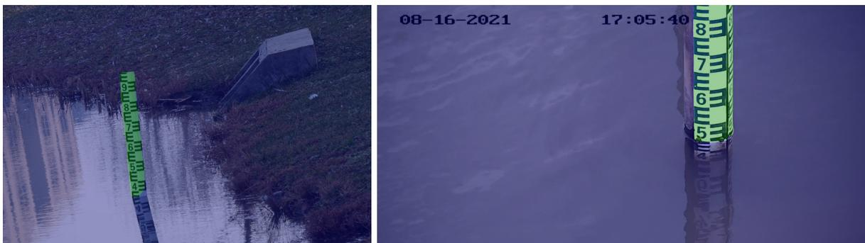
**Figure 12.** Reflection water gauge image segmentation results.
