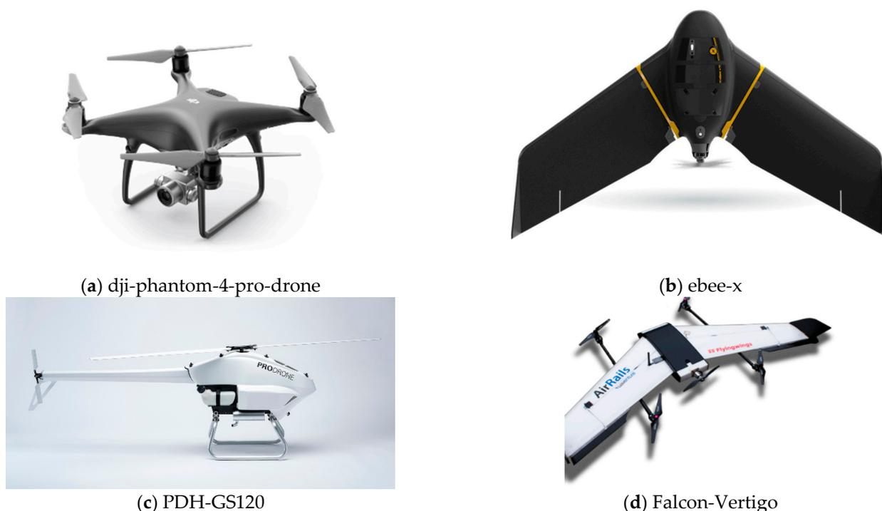
**Figure 6.** (a) multi-rotor <https://www.stickpng.com/img/electronics/dji-drones/dji-phantom-4-pro-drone> (accessed on 17 October 2022), (b) fixed-wing <https://www.sensefly.com/drones/ebee-x/> (accessed on 17 October 2022), (c) single-rotor helicopter <https://www.prodrone.com/products/pdh-gs120/> (accessed on 16 October 2022) and (d) fixed-wing hybrid VTOL <https://www.uasvision.com/wp-content/uploads/2017/02/Falcon-Vertigo.png> (accessed on 17 October 2022).
