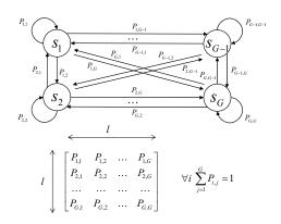
Figure 2. The schematic diagram of the FSMC, which contains G states.
