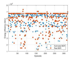
Figure 9. The performance of the proposed DDQN scheme based on the real BER and estimated BER.
