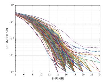
Figure 1. The BER performance for the same MCS system under different simulated UWA channels.
