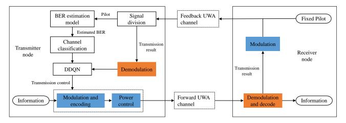
Figure 3. The structure diagram of the proposed AMC system.
