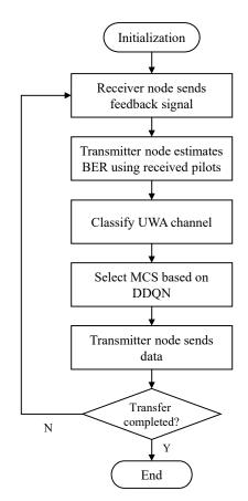
Figure 5. The flow chart of the proposed scheme.
