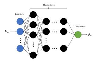
Figure 4. The structure of the proposed DNN for BER prediction.
