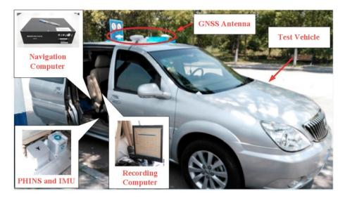
Figure 2. Installation diagram for vehicle-mounted experiment.
