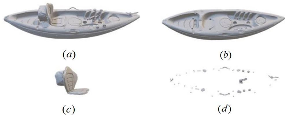
**Figure 12.** Material of the assault boat: (a) main boat body; (b) bottom plate (fiber-reinforced plastics); (c) seat plate (special steel); (d) accessories of the assault boat (copper nickel).
