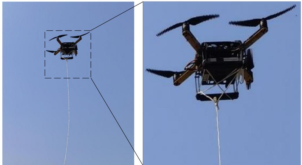
**Figure 7.** An actual experimental attack picture: a nylon cord is fastened to the bottom of the UAV.
