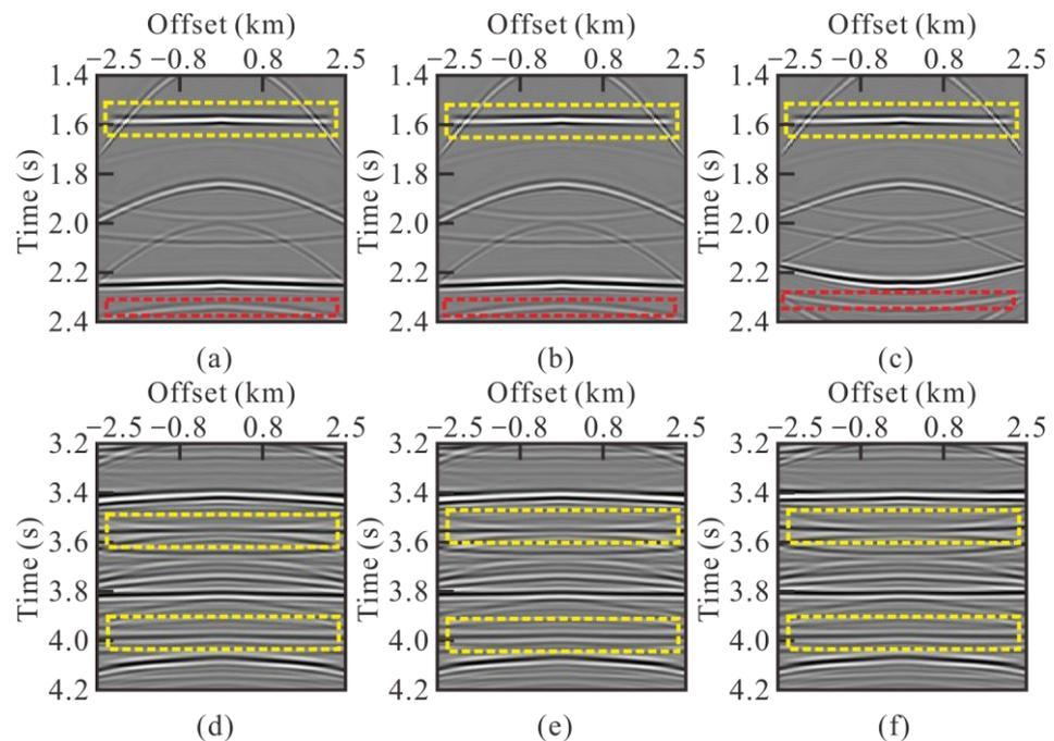
**Figure 7.** NMO comparison results. 1.4–2.4 s: (a) NMO results of the MP velocity, (b) NMO results of the AD velocity, (c) NMO results of the MA velocity. 3.2–4.2 s: (d) NMO results of the MP velocity, (e) NMO results of the AD velocity, (f) NMO results of the MA velocity.
