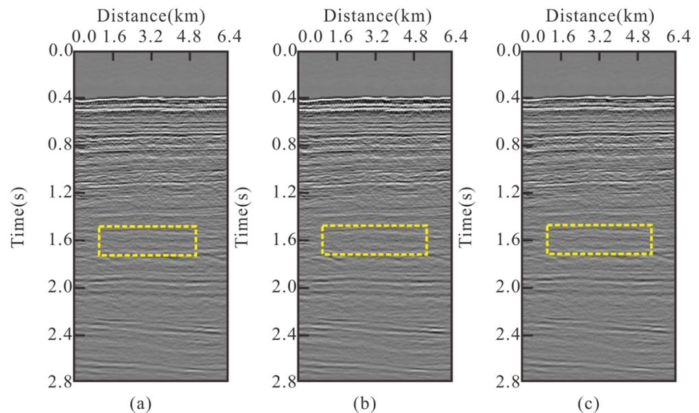
**Figure 10.** Comparison of stacked sections: (a) stack result of reference velocity, (b) stack result of the velocity obtained by control group, (c) stack result of the velocity obtained by proposed method.
