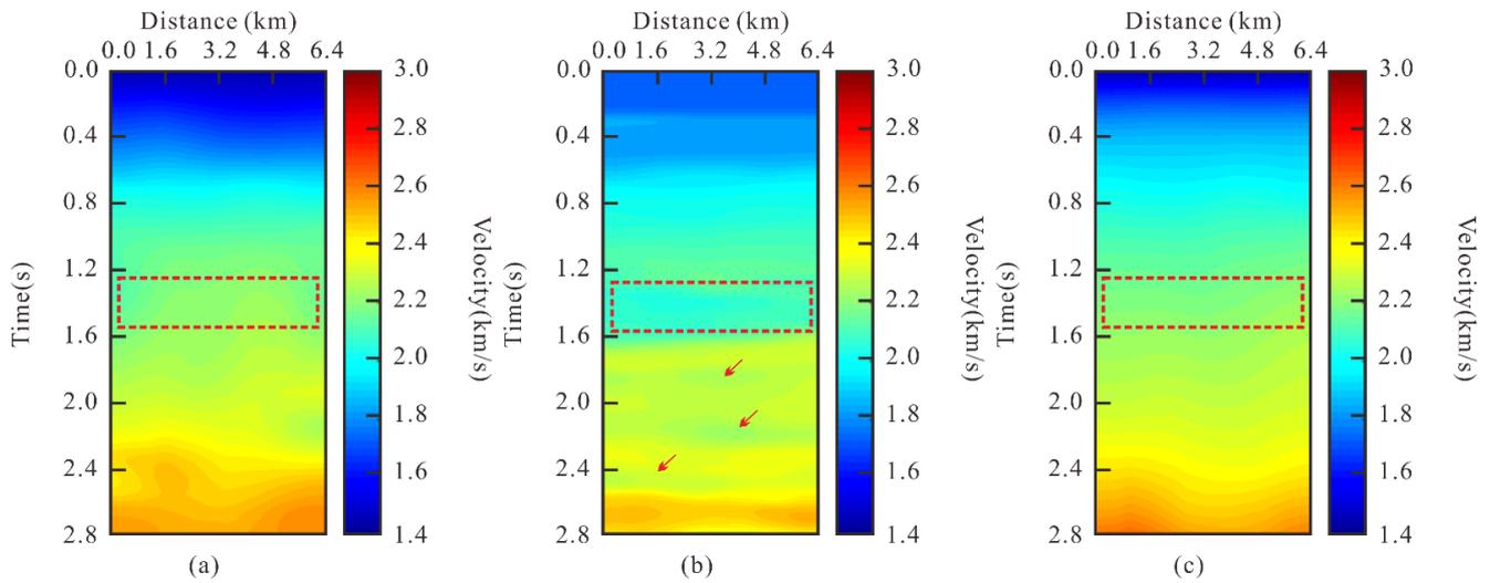
**Figure 9.** Comparison of velocity model: (a) reference model, (b) velocity model obtained by control group, (c) velocity model obtained by proposed method.
