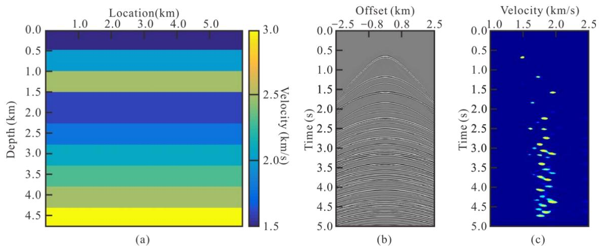
**Figure 4.** Display of synthetic data: (a) Velocity model containing a velocity reversal, (b) CMP record of original data, (c) velocity spectra of original data.
