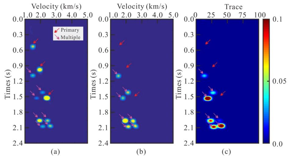
**Figure 2.** A demonstration of the similarity between the original data velocity spectra and the predicted multiple velocity spectra: (a) the velocity spectra of original data. (b) The velocity spectra of predicted multiples. (c) Local similarity spectra.
