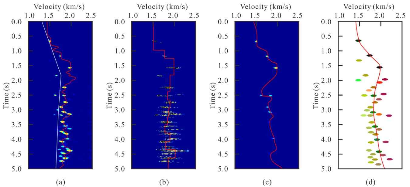
**Figure 5.** Display of synthetic data test results: (a) muting-based strategy (MU), (b) Radon transform strategy (RT), (c) multiple attenuation strategy (MA), (d) proposed advanced method (AD).
