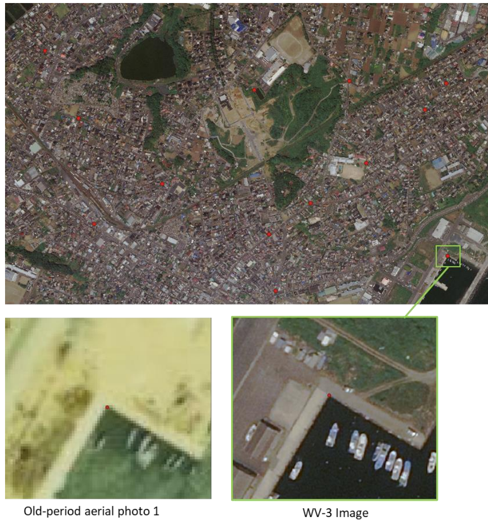
Figure 10. Thirteen GCPs (red points) manually acquired from WV-3 image in Hitachinaka area (top). Enlarged images of old-period aerial photo 1 and WV-3 image are shown with one GCP acquired from each image (bottom).
