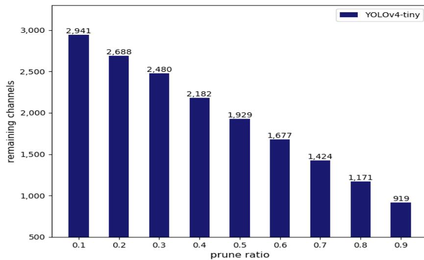
Figure 12. Number of channels remaining in the model with different pruning ratios.
