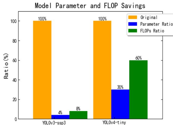
Figure 7. Comparison of the pruned models and the original models on NWPU VHR-10. The blue and green bars are the parameter and FLOPs ratios between the pruned and original models.
