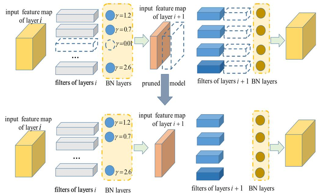
**Figure 2.** Network pruning process. The dotted line in the upper part of the image represents the filter and feature map that the network needs to be pruned, and the bottom part represents the pruned network. When channels with a  $\gamma$  value less than the fixed threshold are eliminated in the current convolution layer, the filters of the next layer in the channel dimension also need to be deleted together.
