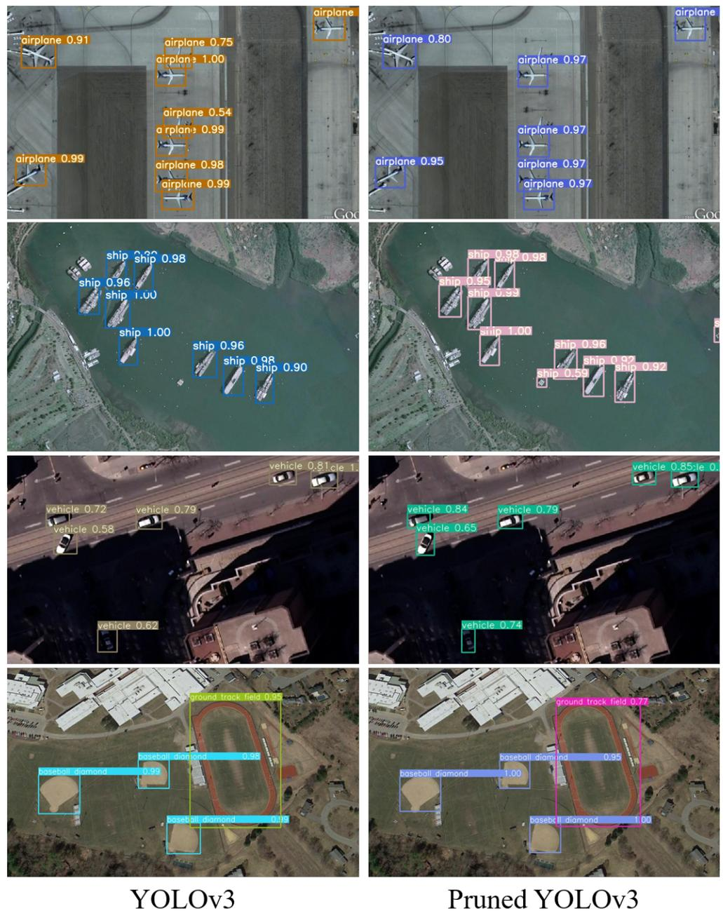
**Figure 9.** Visual detection results of YOLOv3 and the pruned YOLOv3.
