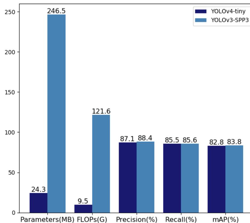
**Figure 4.** Performance comparison of YOLOv4-Tiny and YOLOv3-SPP3 with an input size of  $800 \times 800$ .
