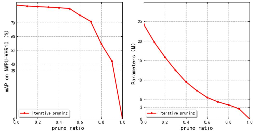
Figure 6. The effects of various pruning percentages with YOLOv4-tiny trained on NWPU VHR-10.
