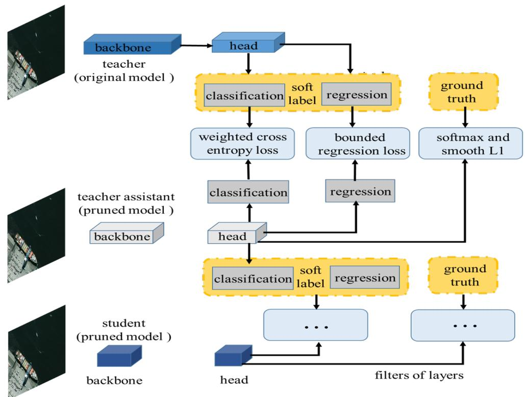
**Figure 3.** Assistant distillation workflow. The original network is used as a teacher, the network generated through intermediate pruning is used as a teacher assistant, and the lightweight network after iterative pruning is used as a student network.
