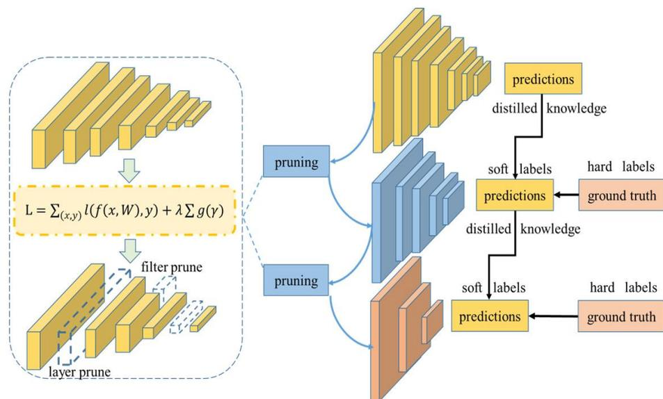
**Figure 1.** Compression architecture based on sparse channel pruning and assistant distillation. The intermediate model retained in the iterative pruning process serves as the assistant model. The precision of the model is restored after pruning by the way of the teacher’s distillation of the assistant and the assistant’s distillation of the student.
