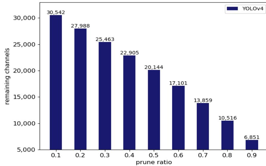
**Figure 10.** Number of channels remaining in the model with different pruning ratios.
