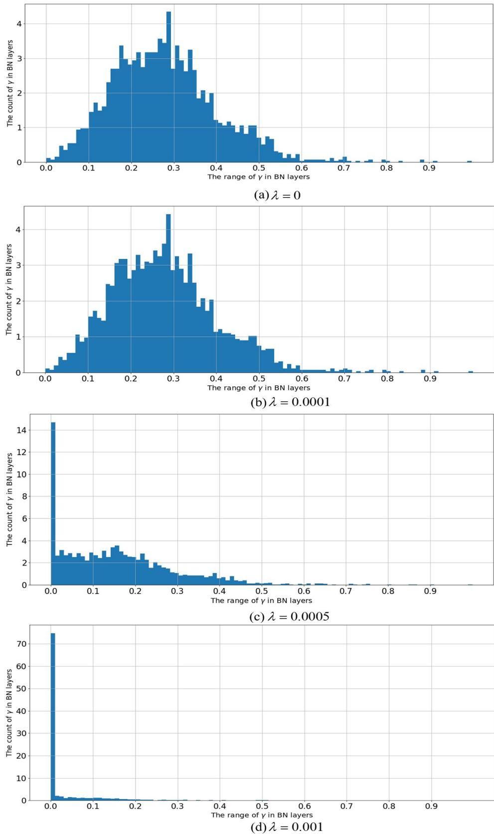
Figure 5. Schematic diagram of the scale factor distribution under different sparse factors.
