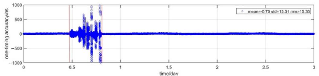
**Figure 6.** BDS-3 RDSS one-way timing accuracy (orbit maneuver state).
