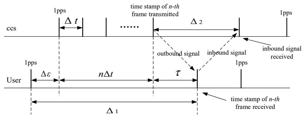
Figure 2. The two-way timing principle.
