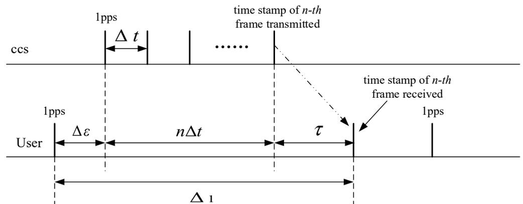
Figure 1. The one-way timing principle.
