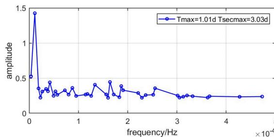
**Figure 8.** Spectrum analysis results of RDSS timing error.
