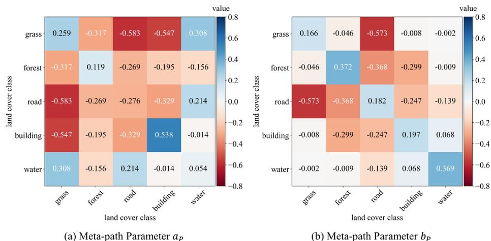
Figure 8. Symmetric meta-path parameters  $a_p, b_p$  in edge calculation. The values are rendered with the color bar on the right, with positive values appearing in blue and negative values in red.
