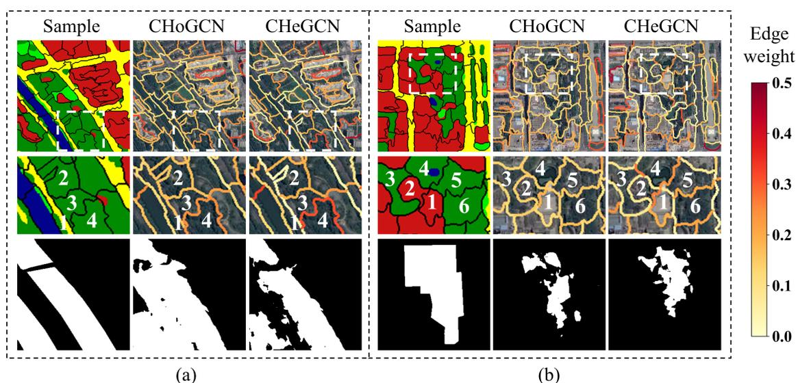
**Figure 7.** Visualization of edge weights among land cover objects and the segmentation results. There are two examples shown in (a,b) and the numbers in the second row denote the index numbers of different nodes. The color bar on the right is used to render edge weights, with higher values making edges redder.
