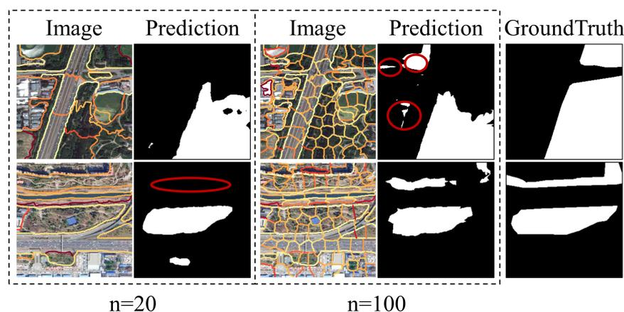
**Figure 10.** Comparison of qualitative results at different segmentation scales. Segmentation results of different segmentation scales are placed on the image. Predicted differences are marked with red circles.
