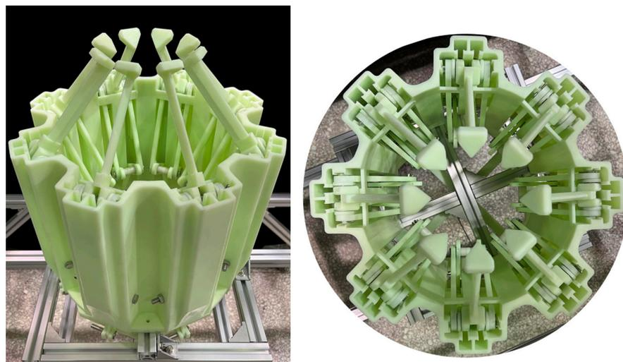
Figure 16. Active part of the deployable docking mechanism.
