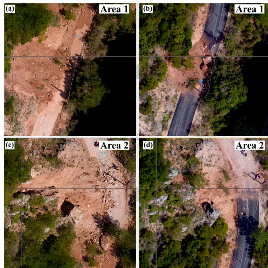
Figure 8. Orthophotos: (a) Area 1 on 11 April 2020, (b) Area 1 on 21 April 2019, (c) Area 2 on 11 April 2020, (d) Area 2 on 21 April 2019.
