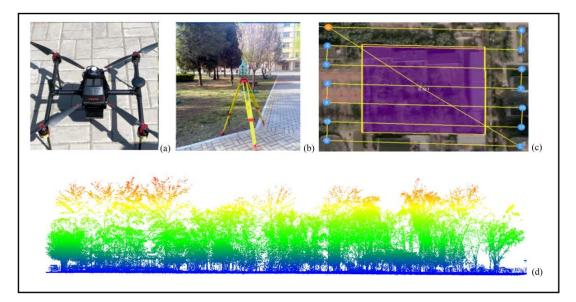
**Figure 2.** (**a**) The UAV, (**b**) The total station with the scanning mode, (**c**) The flight plan and (**d**) Point cloud image.
