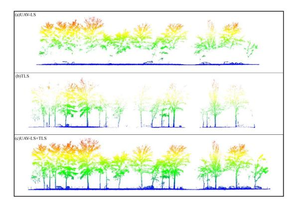
Figure 5. Point cloud data graph combining the TLS and UAV-TLS collections.
