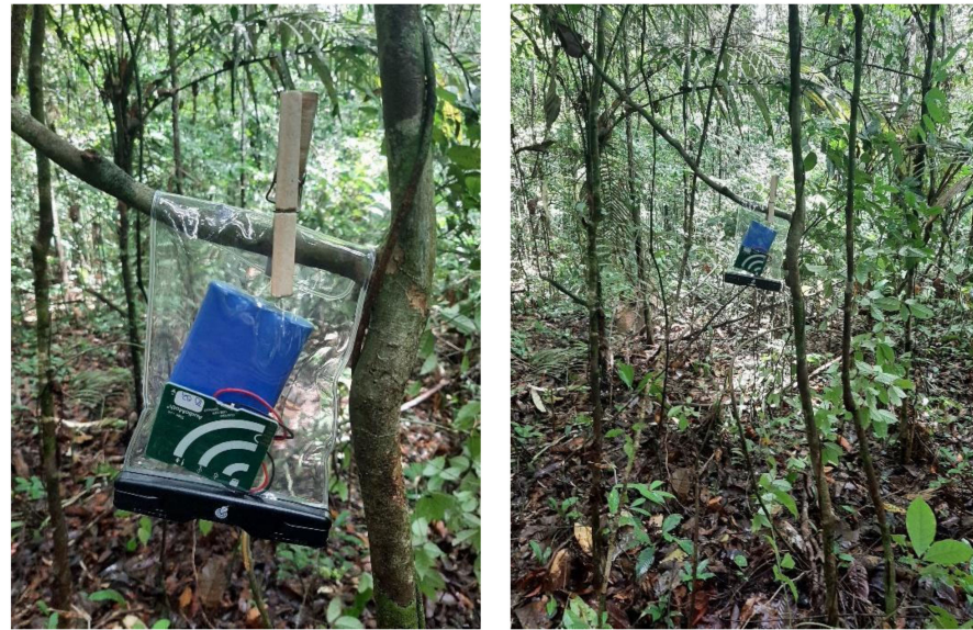
Figure A2. The AudioMoth device, an open acoustic, lightweight, and affordable autonomous recording unit used to monitor the soundscape in Puerto Rico during 2021. The device hardware, which included a lithium-ion rechargeable battery (blue packet in the photo), was placed in a protective waterproof plastic case with a silica packet and then deployed in a tree/vine/shrub at a 1.5 m height.
