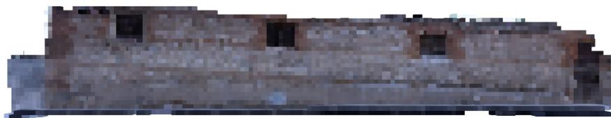
**Figure 18.** Voxelization with a voxel size of 15 cm.
