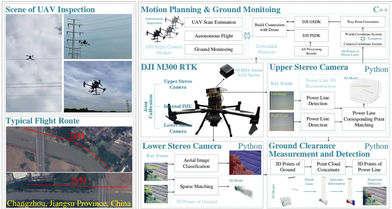
Figure 2. Overall framework of the proposed UAV-based inspection platform.
