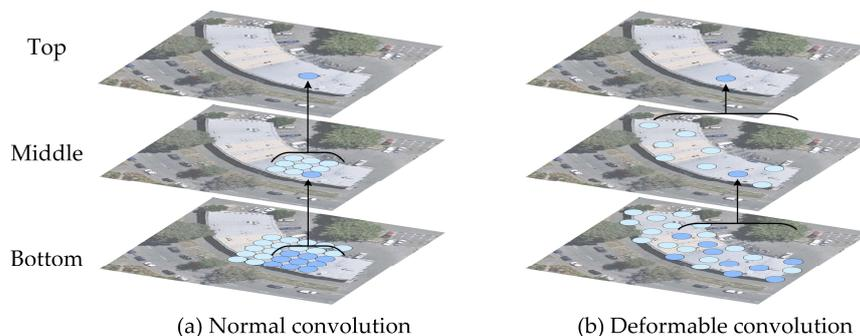
**Figure 5.** Schematic diagrams of (a) a normal convolution and (b) a deformable convolution. From the bottom to the top, the sampling points are fixed in the normal convolution, while the sampling points in the deformable convolution adjust according to the shape of the object.
