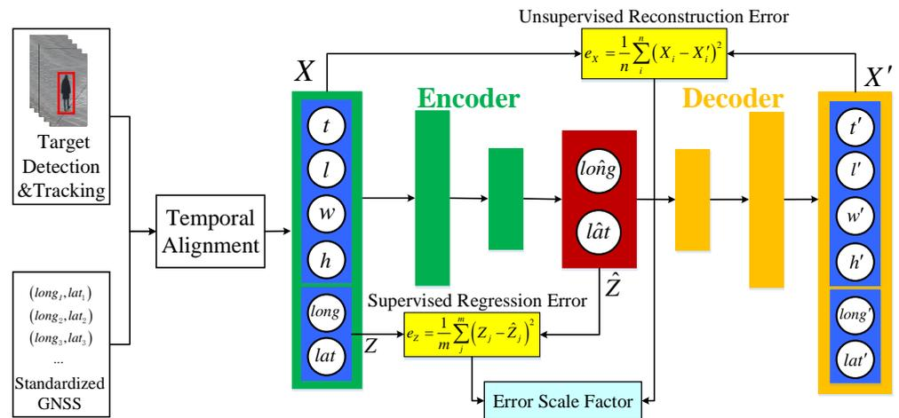
**Figure 3.** Framework of Stage One, with a hybrid stacked auto-encoder backbone.
