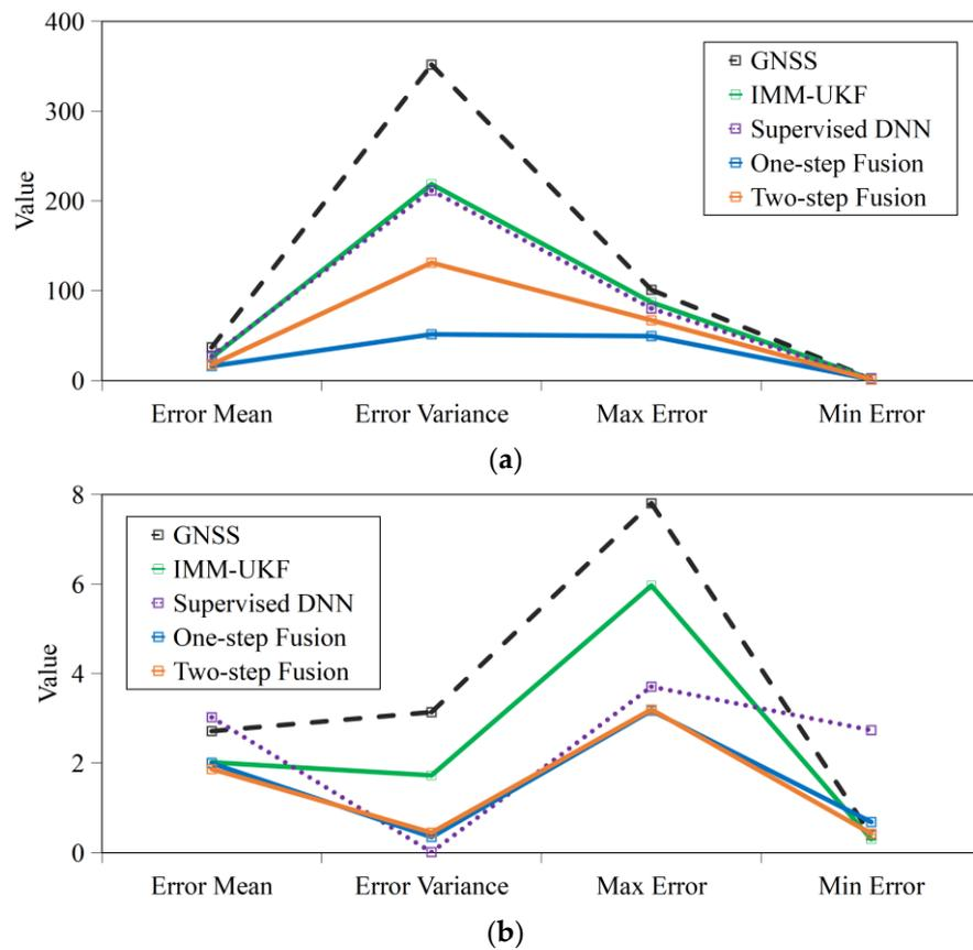
**Figure 7.** Statistical parameters of location errors. (a). Statistical parameters of location errors in Scenario 1. (b). Statistical parameters of location errors in Scenario 2.
