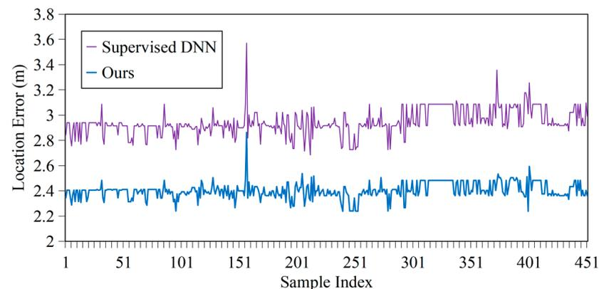
**Figure 15.** Location error curves when GNSS is denied in Scenario 2.
