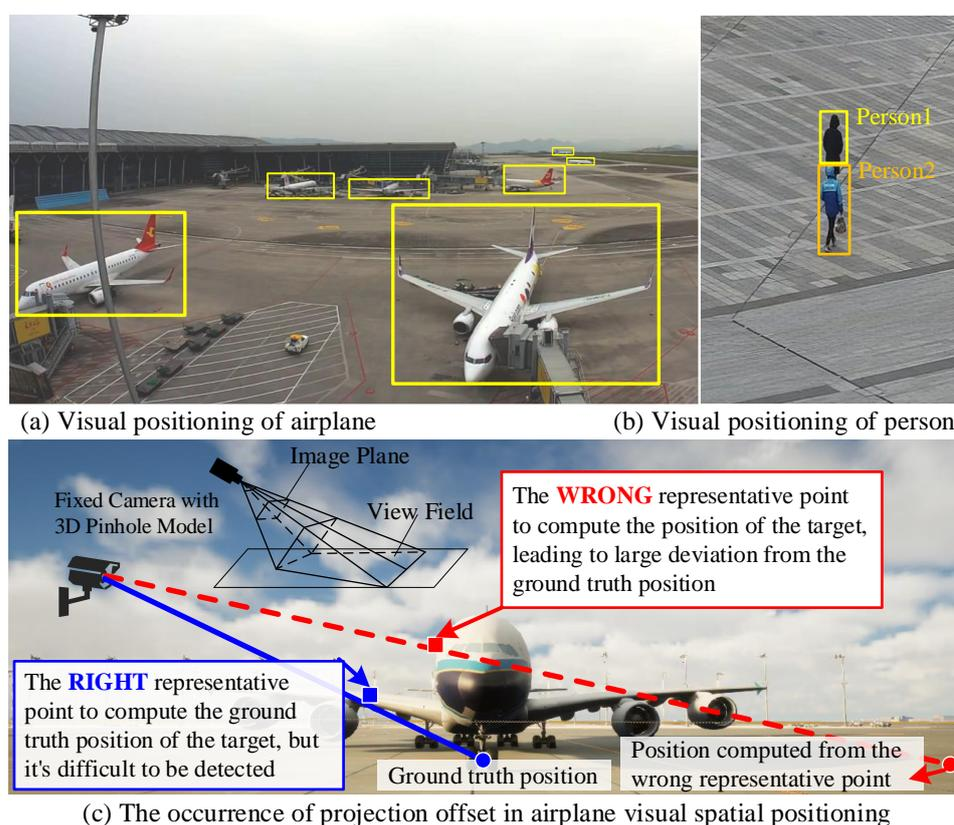
**Figure 1.** (a,b): The difficulty of choosing visual representative positioning feature points. (c): The occurrence of projection offset in traditional visual spatial positioning methods, produced by the pinhole-based 3D camera model if choosing a wrong representative positioning feature point, which is difficult to be overcome in existing visual positioning methods.
