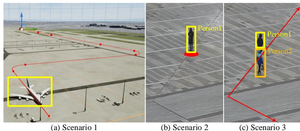
**Figure 5.** Experimental scenarios. (a) In Scenario 1, the simulated airplane taxed along the taxiway (red). (b) In Scenario 2, the target Person 1 stood still at a fix point (red). (c) In Scenario 3, the target Person 1 walked back and forth along a polyline (red) where some occlusions occurred between pedestrians. The yellow and orange boxes represent the object detection bounding boxes.
