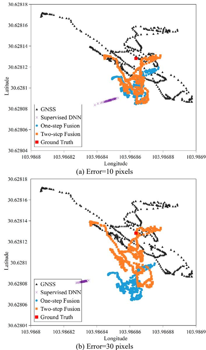
**Figure 12.** Location distributions with different errors of image bounding box tensors in Scenario 2.
