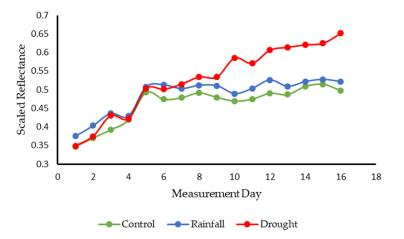
**Figure 10.** Spectral change observed at 680 nm for each group. Note the continued increase observed in the drought group for the duration of the measurement period. Measurement Day represents days on which measurements were collected rather than a consecutive time period.
