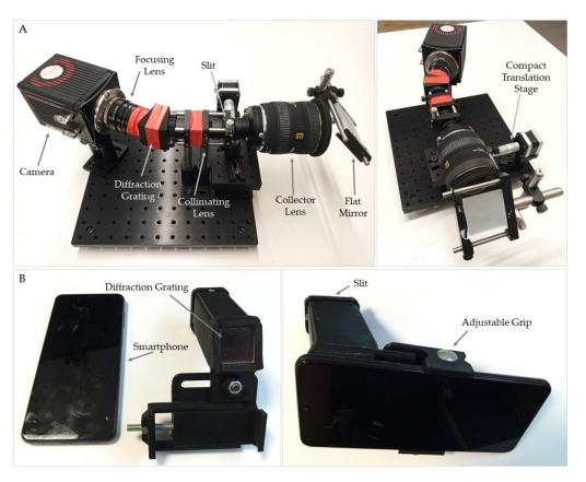
**Figure 1.** Low-cost hyperspectral imaging instrumentation utilised within this research. (**A**) shows the semi-portable Low-Cost High-Resolution instrument. (**B**) shows the ultra-low-cost Hyperspectral Smartphone instrument both before connection with a smartphone (left) and after connection and alignment of the spectral components with the built-in smartphone camera optics.
