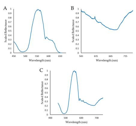
**Figure 5.** Example dataset combination. (**A**,**B**) show the individual spectral responses captured by the Hyperspectral Smartphone and the Low-Cost High-Resolution instrument, respectively. (**C**) shows the full dataset after combination. Note, the relative intensities remain accurate after combination.
