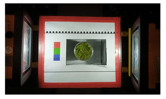
**Figure 3.** A sample of Sphagnum moss ready for image capture using the hand-held Hyperspectral Smartphone and the in-scene reference card.
