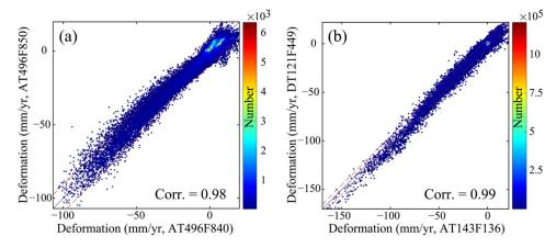
**Figure 7.** Comparison between the results obtained by (a) ALOS-1/PALSAR AT496F840 and AT496F850 data, and (b) the Sentinel-1 AT143F136 and DT121F449 data. The red dotted lines denote the value three times the root-mean-square error.
