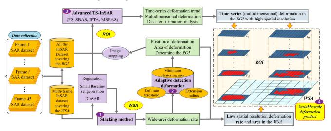
Figure 1. Flowchart of the method for the variable-scale monitoring of deformation in a wide area.
