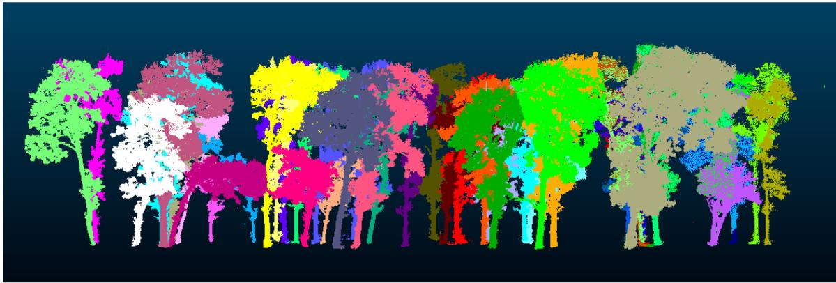
**Figure 5.** Study area from a terrestrial laser scanning point cloud taken using the FARO Focus 3D X330. These trees were placed back in after the point cloud was divided into single woods. To distinguish the different trees, they are given different colors.
